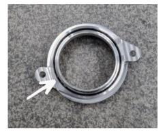
Step 15 Install the included O-ring on the aluminum turbo inlet joiner.
