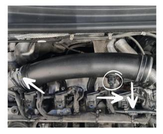
Remove the engine cover, grab the corners and gently lift it upwards.
