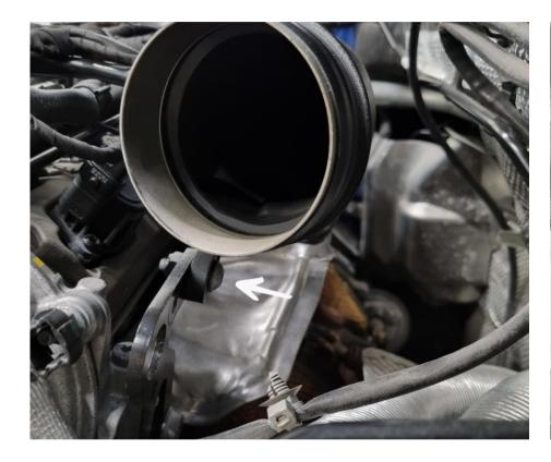
Remove 1x Torx T30. Remove the inlet pipe from the car.
