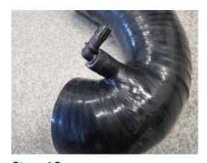
Step 19 Install the included 90 degree elbow connector and secure it with an included hose clamp.
