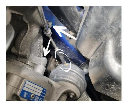
Remove 2x Torx T30 (one holds vacuum pipe and one secures turbo inlet to turbocharger) and loosen the small hose from the wastegate. Remove the small metal pipe and rubber hoses from the car. This will be replaced with the included 4mm silicone hose, 60cm long.
