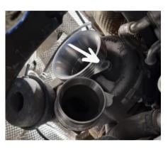
Step 16 Install the aluminum turbo inlet joiner
