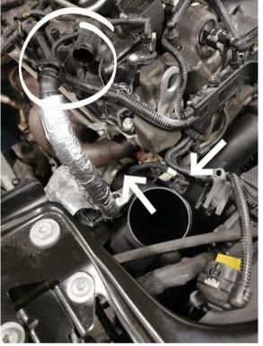
Unclip the heat protection blanket and disconnect the wastegate electrical connection underneath. Then disconnect the electrical connection in the valve cover breather hose and unclip the wires from it.
