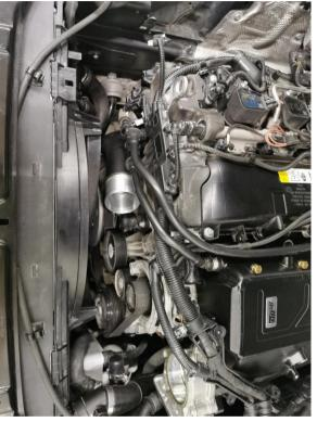
Remove the c-clip from OE pipe by prying of the plastic retainer. Then transfer the OEM sealing ring and install it and the c-clip to the do88 performance charge pipe. Ii you had a sealing ring included in your pipe kit, please use that sealing ring instead.
