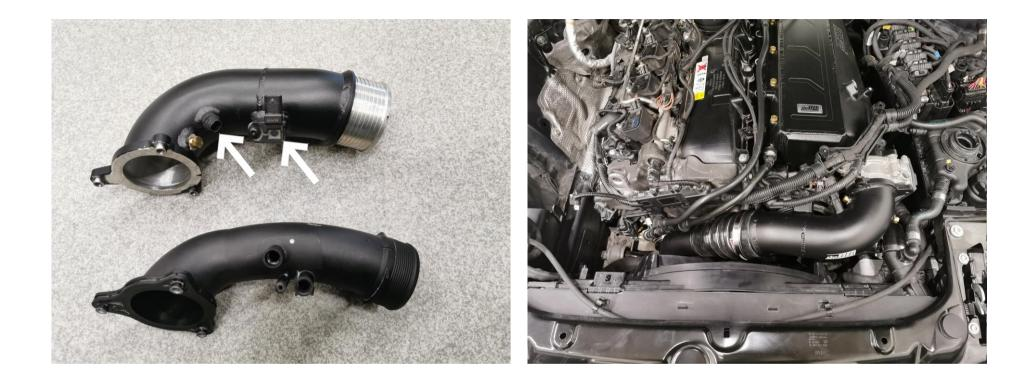
Transfer the sensors from the OEM pipe to the do88 performance pipe. Secure with included M6 Screw.
