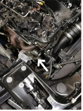
Disconnect the three electrical connections marked on picture, two in the charge pipe and one from the valvetronic motor. Now remove the 3 x T30 screws holding the charge pipe to the throttle body.
