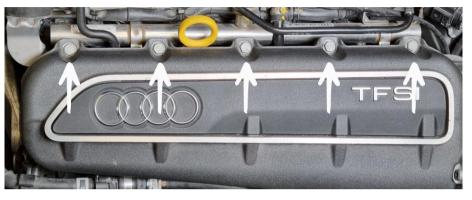
Step 13 Remove 1x 10mm hex screw underneath the intake manifold. Step 14 Remove 5x 10mm hex screws.
