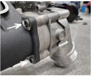
Step 20 This Step is only for install of do88 throttle body spacer (CP-130)
