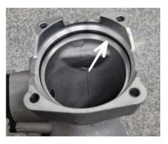
Step 23 Remove the O-ring from the OEM cast elbow and install it in the do88 charge
