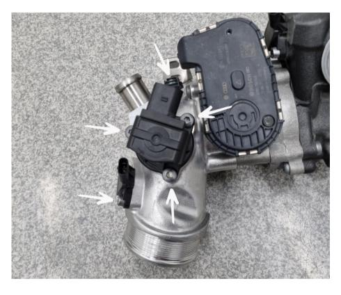
Remove 1x Torx T30 screw from the sensor and 3x Torx T30 screws from the BOV. Remove the rubber bushing for the engine cover.
