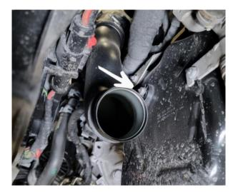
Step 5 Remove 1x 10mm hex screw to the charge pipe bracket.
