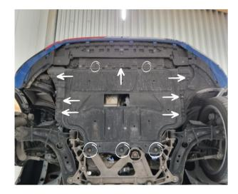
Remove 3x Torx T45 and 7x Torx T25. Use a flat head screwdriver to separate the plastic tabs and remove the plastic cover underneath the car.
