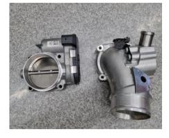
Step 22 Separate the cast elbow and throttle body.
