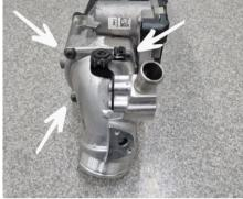
Step 17 Remove 3x Torx T30 screws.
