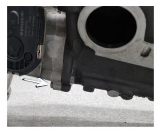
Step 21 This Step is only for install of do88 throttle body spacer (CP-130)
