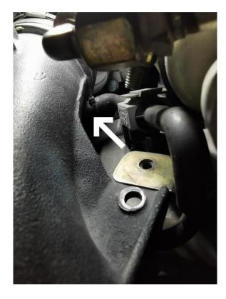
Now pull the charge pipe gently back until it loosens from the throttle body. Then disconnect the vacuum hose from the charge pipe before you remove it entirely.
