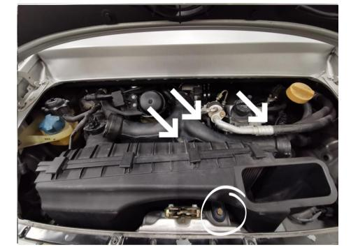
Remove the hoses from the cold side of the intercooler to the charge pipe (2pcs). All hoses ends have clips.
