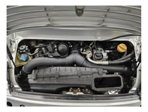
Start by tighten the throttle body hose and then re-install air temperature sensor. The AC-hose clip is secured with included M5 screw. Re-use the 10mm Hex for the two charge pipe mounts. Connect the vacuum line and breather hose, secure with included clamps.
