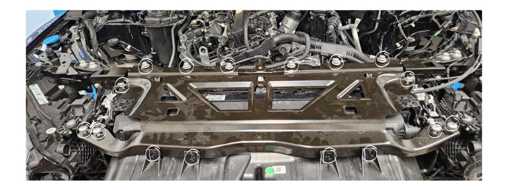
Remove 4x Torx T40 screws / 2x T30 screws / 6x Hex 13mm screws / 4x plastic clips. Then remove the large bracket on top of the radiator.
