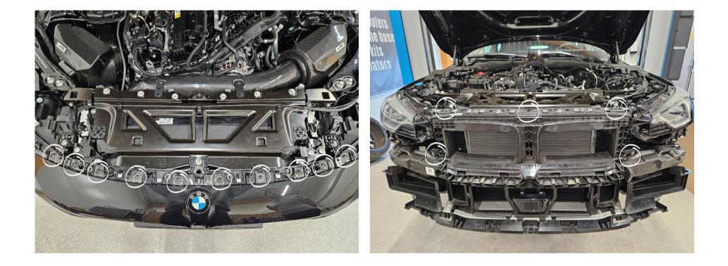
Remove 10x Torx T30 screws from the top of the bumper. Then remove the bumper.
