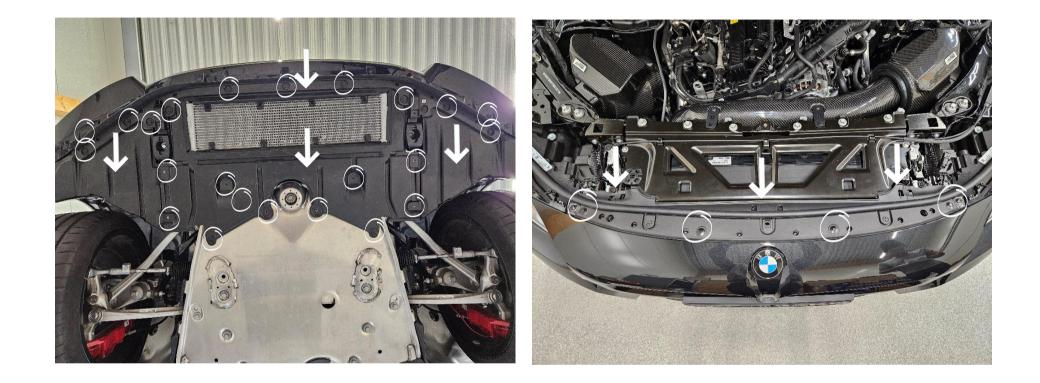
Remove the front spoiler lip, 2x splash guards and plastic undertray by loosening 31x 10mm hex screws.
