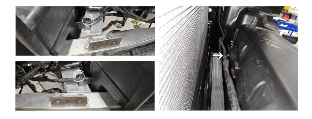
Unclip the wiring harness shows on the photos. Also disconnect cable connectors for the radar unit, temperature sensor (upper grille air guide), 2x horns, 2x airbag sensor (each end of the bumper bar).
