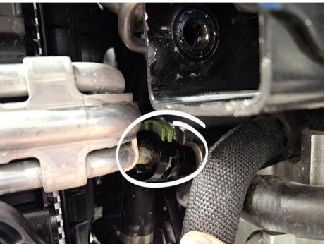
Pre-fill the do88 transmission cooler (use oil according to manufacturer specifications). Then cap the connections with the included caps to prevent oil leakage during installation.
