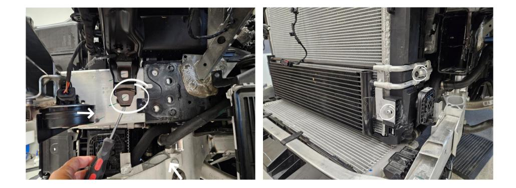
Remove the bumper bar. You will need to pry the marked brackets outwards to let the guide pin pass underneath it.
