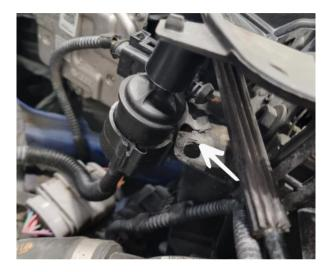
Mount the gearbox breather previously removed from the air filter box on plastic tab underneath radiator support bar.
