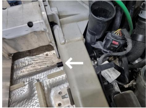
Underneath each intercooler inlet tank install the included brackets.
