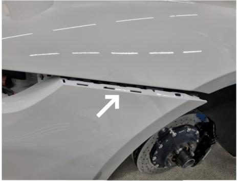
On both sides remove  $2x \, Torx \, T30$  and disconnect  $1x \, cable$  connector marked on photo.
