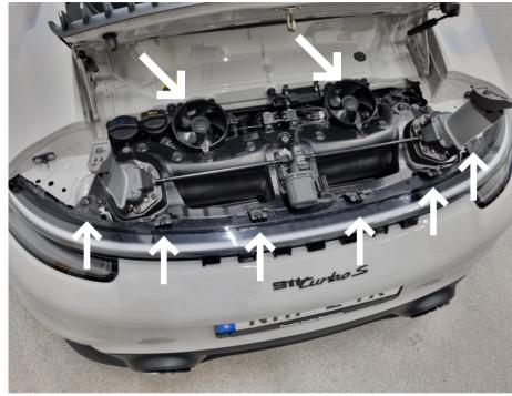
Remove 3x Torx T30 screws and disconnect the brake light cable connector. Then gently pull this panel backwards and lift it straight up. Be careful not to damage the paint around the spoiler mechanism.
