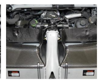
Gently lift the intercooler package into the car, start with the throttle body hose, then into the center rubber grommets.
