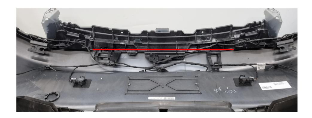
Inside the upper parts of the rear bumper disconnect the cables from their original position and relocate them behind the plastic tabs on the marked area on the photo below. Fasten the cables with the included zip-ties.
