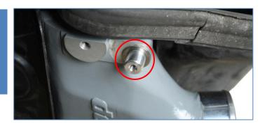
Install both intercoolers in their support frames and then fasten 19. them by installing 4pcs large washers and 4pcs M6x10 hex head screws in each bushing position on each intercooler according to picture. Use thread locker and tighten loosely.
