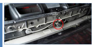
9. Loosen the intercooler outlet hose (upper) from intercooler on both sides by prying out the quick coupling lock clips with a flat screwdriver about 10mm.
