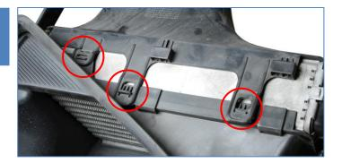
Remove the 4pcs metal C-clips from each intercooler that holds it in the support frame by prying the C-clip out of the groove in the original intercooler with a flat screwdriver.
