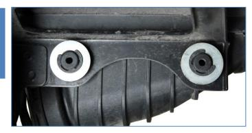
**16.** Remove the ambient outlet air guides from the intercoolers.
