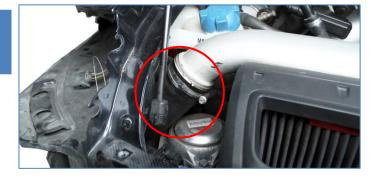
14. From both intercoolers, remove the intercooler inlet air guide by unclipping the 6 plastic fasteners that holds it to the outlet air guide with a flat screw driver.
