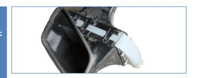
Install two included aluminium bushing holders with one large flat 18. washer under each bushing holder on each intercooler. Use the supplied thread locker on the threads, torque loosely with a plier.
