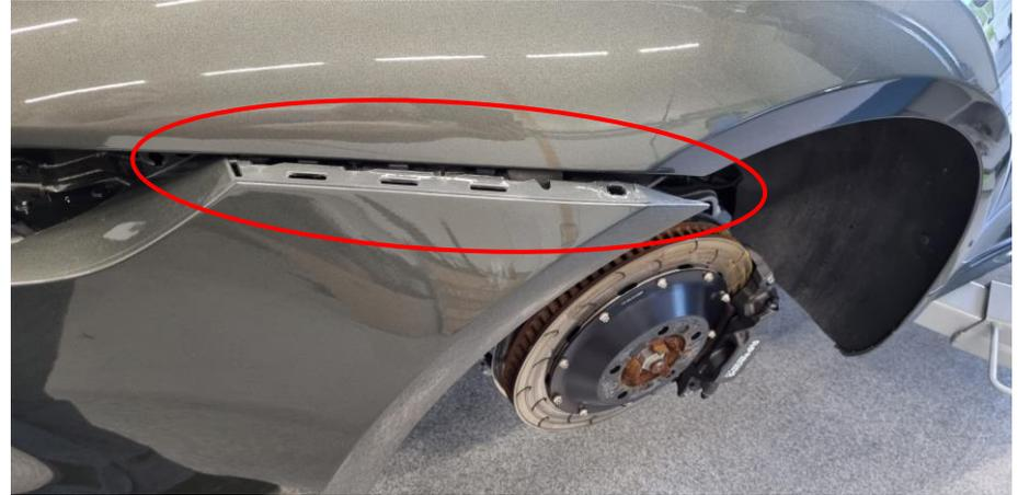
**19.** Remove the spoiler mechanism. 4x Torx T45 and 1x cable connector.
