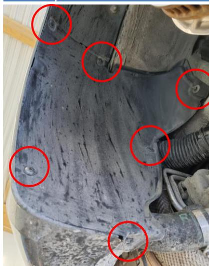
**13.** Remove 8x Torx T30 located in the bottom of the rear bumper cover. For installation purpose, note that the two in the middle has different threads.
