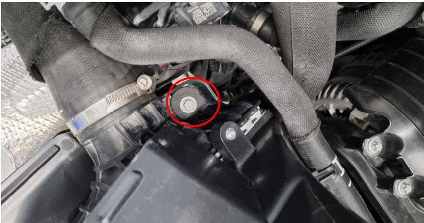
**22.** Remove the two clips and washers from the center intercooler bracket. It is a tight space to reach the front clip but can be done using two screw drivers.
