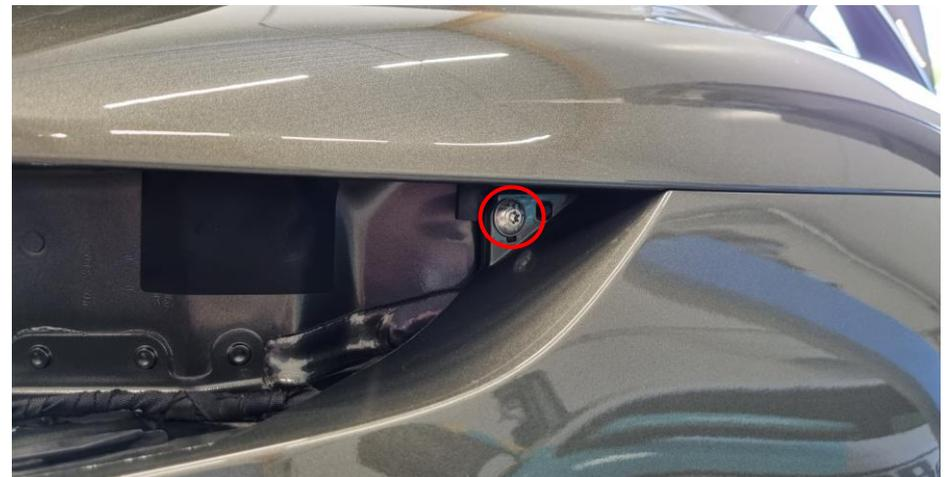
**17.** Disconnect the left and/or right cable connectors for the rear bumper. Number of connectors depends on equipment installed in the car.
