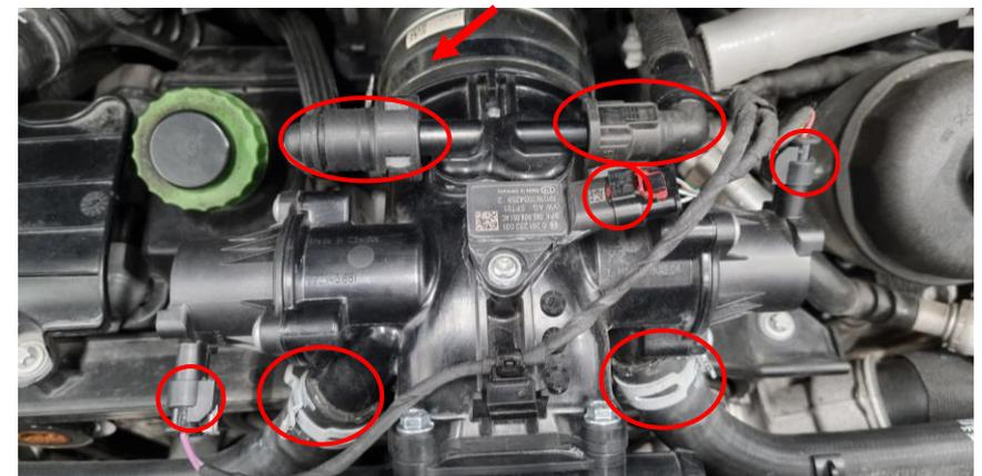
**25.** Loosen hose clamps and then remove the intercooler inlet hose on both sides. Then lift out the intercooler from the car.
