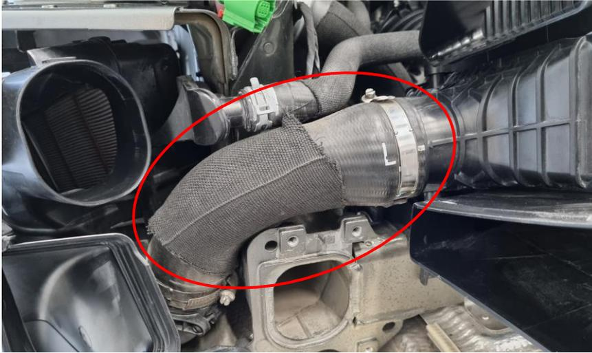
**26.** Remove both plastic intercooler side brackets. Push the plastic locking pins rearwards using a 10mm hex socket as on the photo.
