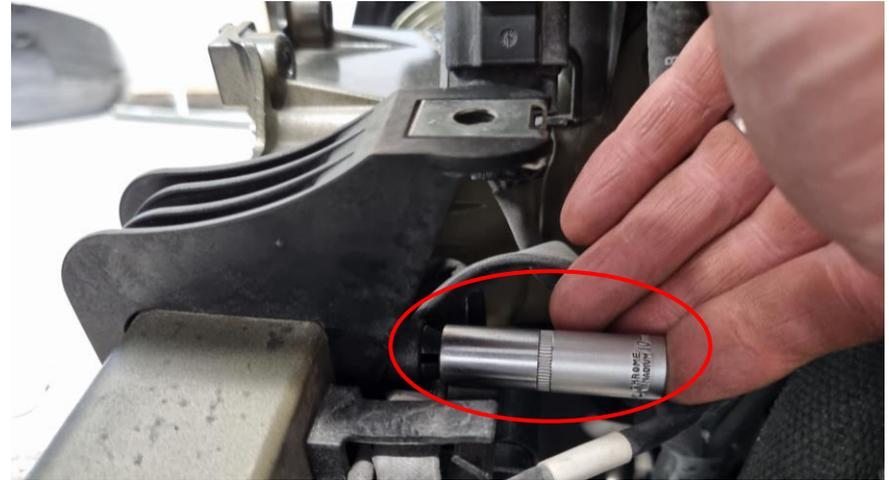
**27.** Remove the intercooler outlet hose connection body. 4x screws. Also gently remove the square O-ring.
