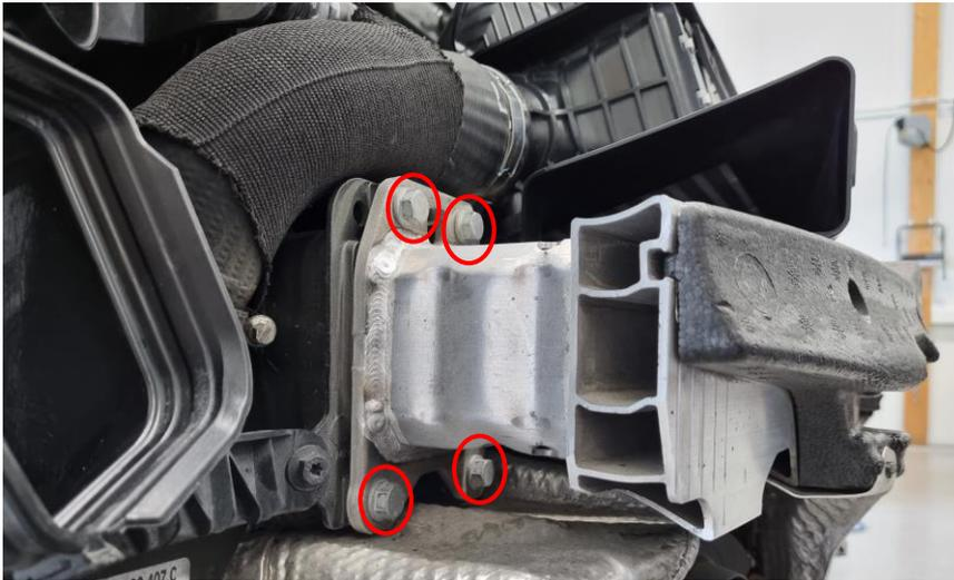
**23.** Remove 1x Hex 10mm screws on each side of the intercooler.
